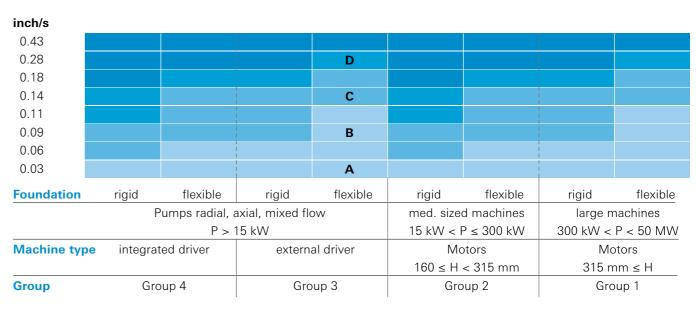
DIN ISO 10816: Mechanical vibrations – assessment of the vibrations of machine through measurements on no rotating parts. Vibration velocity (rms) 10 – 1000 Hz, n > 600 min<sup>-1</sup>, 2 – 1000 Hz, n > 120 min<sup>-1</sup>
